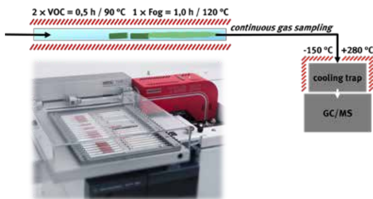
Illustration 3: schematic material test procedure according to VDA guideline 278
