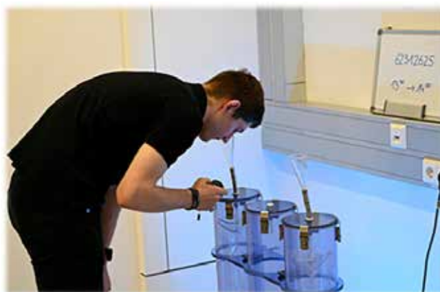
photograph 1: odor assessment according to ISO 12219-7 from bags using a presentation device
