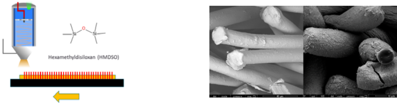
Figure 8: Plasma nozzle process schematic (left), comparison of the uncoated and coated flock fibres (right).
