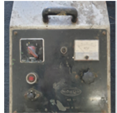
An Electrostatic Generator Mod. TE1 (Still working, owned by M/S Qualplast)
